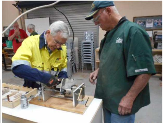
This interesting contraption has been built from scratch by John Gardiner. It uses a Dremel as a router to cut enhancements and is suitable for small cylindrical items such as pens.
