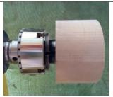
1. Mount blank on screw chuck. True to 120mm dia. x 70mm thick.
