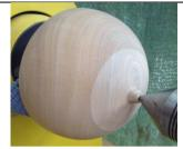
4. Remount bowl using chuck & tailstock centre. Remove waste spigot & sand.
