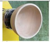
3. Reverse & mount on scroll chuck. Turn & finish inside shape.
