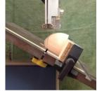
3. Third cut: Tilt table to 30 degrees setting. Place 12mm spacer against fence & cut. Repeat with other half.
